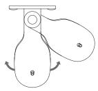
Attention: After changing the position, ensure that the fixing screw is still tight.
