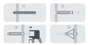
Ensure that neither the screw nor the dowel spins freely in the hole. Do not fix to hollow brick. If you do not feel confident or have not understood the contents of this manual, do not fit the Gecko wall mount and seek the help of a professional.
